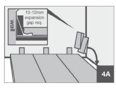
It is critical to keep the first three rows straight and square as their alignment will affect the rest of the installation.
