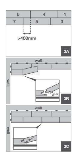
You can tap the long side of the plank into the groove by using a professional tapping block. The planks should not be joined by a single tap. To avoid damaging the planks, you must tap them together gradually without applying excessive force.
