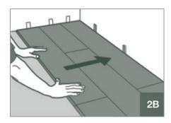
Always ensure that the end joints are randomly staggered at least 450mm apart.
