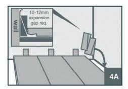
It is critical to keep the first three rows straight and square as their alignment will affect the rest of the installation.
