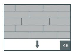
Always ensure that the end joints are randomly staggered at least 400mm apart.
