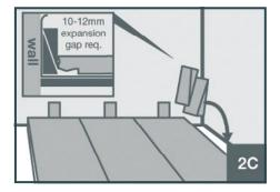
Position the **SHORT SIDE** of the next plank to be installed at angle of 20-30° to the first plank already installed. Move the plank gently up and down and at the same time exert forward pressure. The planks will automatically click into place.
