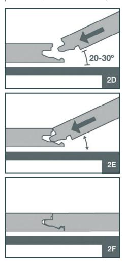
Repeat the same process for the next 3-4 planks and then start the second row. Ensure the long sides of the planks make a straight line.
