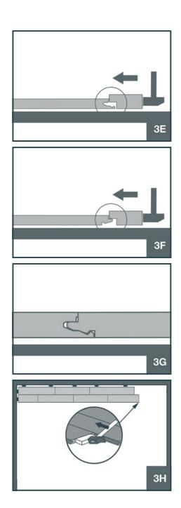
DO NOT TAP THE LONG SIDE OF THE PLANK AT ANY TIME AS IT WILL DAMAGE THE LOCKING MECHANISM.
