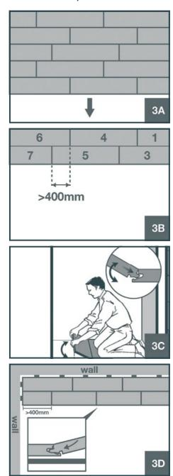
Place the long side of the plank into the first row at angle of 20-30°, the planks will automatically click together. Engage the short side tongue of the new plank into the groove of the first plank of the second row at a 20-30° angle. Push the long side tongues of the new plank at angle of 20-30° into the groove of the planks of the first row. Move the plank gently up and down and at the same time exert forward pressure. The planks will automatically click into place.
