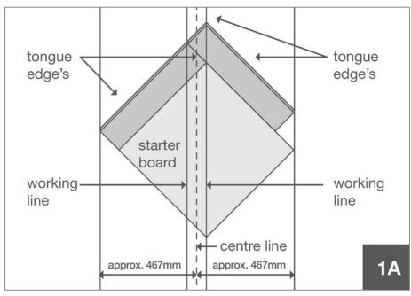
• Set the first right-tongue plank to the right-hand side of the starter board. The grooved side snug must be towards the starter board and the tongue side facing out towards the room. Please make sure the upper butt ends are aligned with the centre line. Press the right-tongue plank down to the subfloor over the **Moisture Barrier Membrane**.
