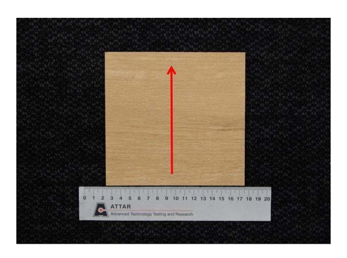
Figure 1: LVT Symphony 2.5mm vinyl plank stair tread Arrow indicates direction of testing
