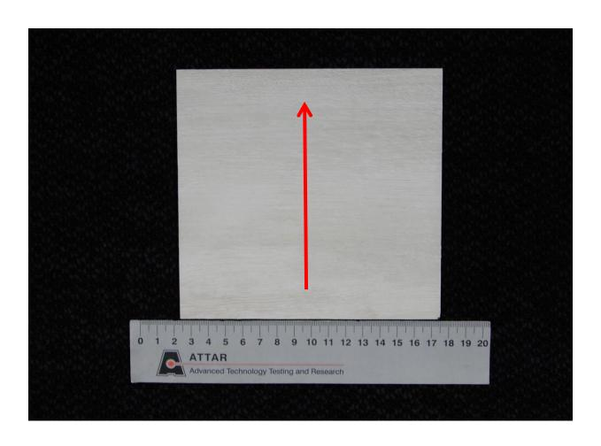
Figure 1: LVT Symphony 4.5mm vinyl plank stair tread Arrow indicates direction of testing
