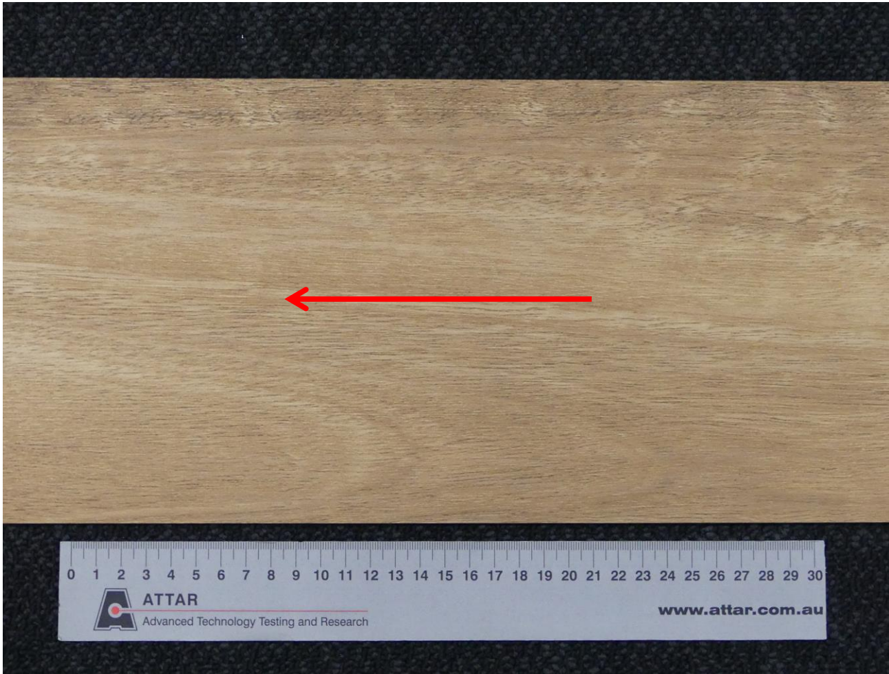
Figure 1: LVT Tahoma 2.5mm Vinyl Plank Arrow indicates direction of testing
