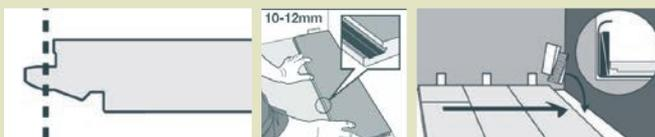
**4. Completing the first row** Place the final plank face down. The distance to the wall must be 10-12mm. Mark where the plank is to be cut. Place the plank face down on the work surface and cut to size using a circular saw. If you are using a hand saw, ensure that it is fine toothed and cut the plank face up.
