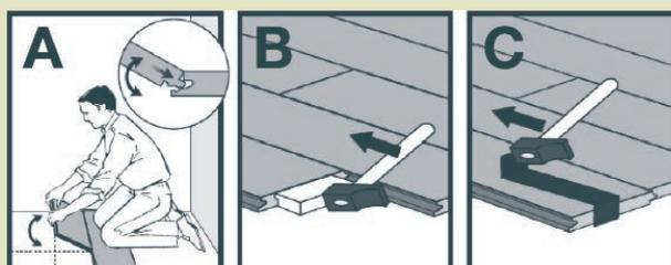
**7. Laying the last row** Measure and cut the plank. Leave 10-12mm gap to the wall.
