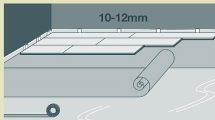
**3. First row** Start installation of the planks in the left-hand corner, tongue-side against the wall. Begin the first row with a whole plank. First saw off the tongue on both long and short sides. Put the plank with sawn off sides against the wall. Put spacers between the planks and the wall. Make sure the expansion joint is 10-12mm from the wall.
